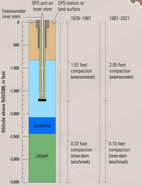
About 370 ft of Evangeline aquifer sediment below the extensometer anchor depth
