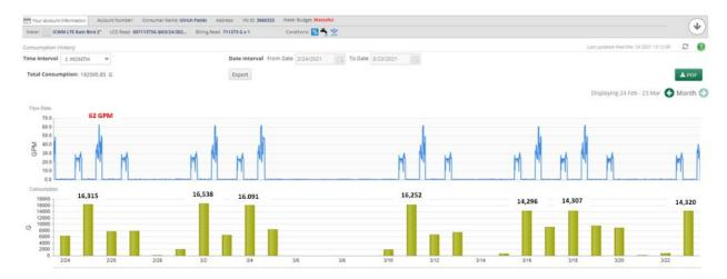
By looking at this schedule, we are certain that the high usage is not due to a leak, but instead scheduling. According to the available report in the Rainbird system, Ulrich Intermediate has used 192,595 gallons between 2/24 and 3/23/2021 (6,420 GPD or the equivalent of running 2.5 hours daily). Based on the system, these were scheduled and not manual run times.
