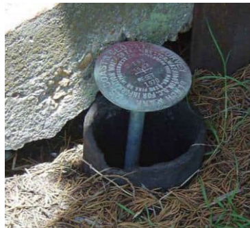
Figure 35: Impacted Vertical Survey Marker (in Louisiana) due to Subsidence of the Surrounding Area xxii
